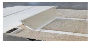
2) Align one of the small side panels in the left groove of the face plate and fasten with provided screws. Duplicate the other side panel.
